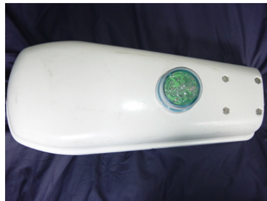
Photo 2-3 - PECU housed on a streetlight
