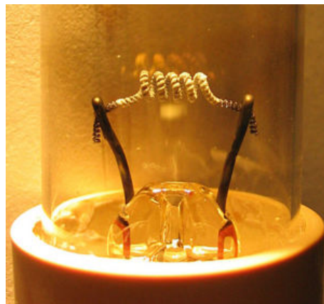
Photo 1 - Close-up of the filament on a low pressure mercury gas discharge lamp showing white thermionic emission mix coating on the central portion of the coil.
